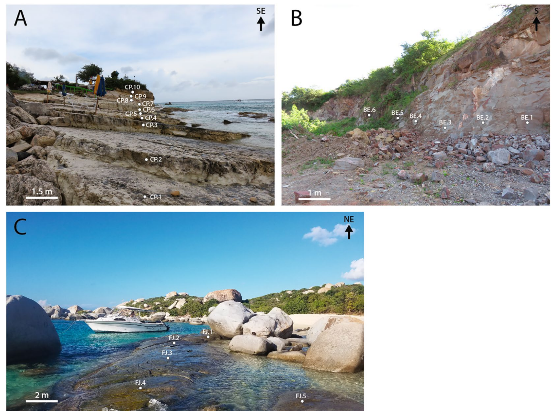
Figure 4. Example of sampling locations in (a) limestones sequence of Cupecoy Beach, in Saint-Martin (sampling location: CP); (b) Andesite of Bental Carry, Antigua (sampling location: BE), and (c) Granodiorite containing mafic enclaves of Fallen Jerusalem, British Virgin Islands (sampling location: FJ).
